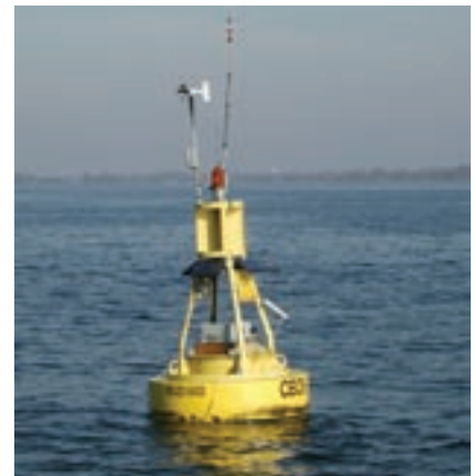
Automated moorings can be equipped with sensors to continuously monitor the temperature and salinity of the water column. The corresponding optical properties can be related to the constituents of the water, including phytoplankton and dense HABs.
